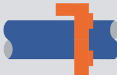
Step 1: Cold-Cut & Bevel the line
