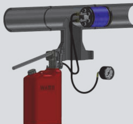
Step 4: Hydrotest all new welds on the fitting and pipe
